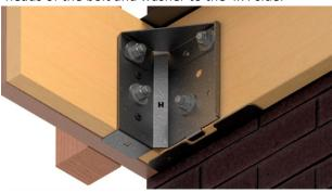
STEP 14: Use 3" width galvanized flashing along the length of the ledger board.
