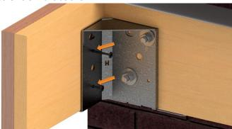
STEP 12: Fasten 4x4 handrail post with temporary toenailing or clamps. Drill through rim joist and 4x4 post allowing the corner bracket to act as guide.
