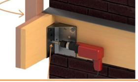
**STEP 13:** Bolt the rim joist assembly together with the heads of the bolt and washer to the 4x4 side.
