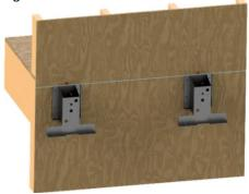
STEP 3: Fasten the H1-GQ bracket into position with 4 screws or nails.
