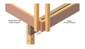
**<u>STEP 4:</u>** Drill, using each bolt hole in bracket as guides, through all lumber with a minimum  $\frac{1}{2}$ " hole for  $\frac{1}{2}$ " bolts or  $\frac{5}{8}$ " hole for  $\frac{5}{8}$ " bolts.
