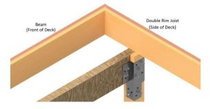
**STEP 2:** Place the H2-GCB bracket flush against corner, ensuring the bracket is flush along the bottom of the rim joist and beam (Optional: Can use screws or nails to temporarily hold in place).
