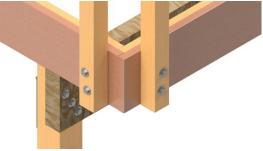
**STEP 6:** Torque per recommended wood council specs. Bolts are ½" diameter minimum. A307 bolts 5/8" thick should be torqued to 73 ft./lbs. A 307 bolts ½" thick should be torqued to 37 ft./lbs.
