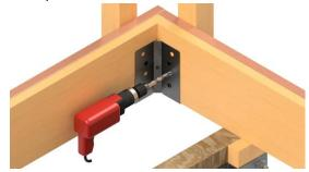
**<u>STEP 5</u>**: Installing bolts through the outside, fasten them inside the deck with code approved fasteners.
