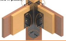
STEP 5: Cut 4x4 handrail posts and toenail or clamp them so that they align with the bolt holes on the bracket side flanges.
