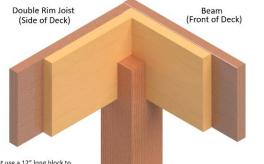
For Single Rim Joist use a 12" long block to permit proper frame spacing.
