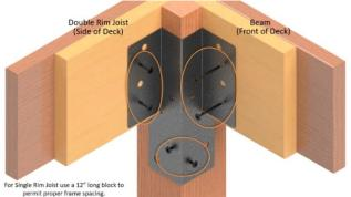
STEP 4: Cut 4x4 handrail posts and toenail or clamp them so that they align with the bolt holes on the bracket side flanges.
