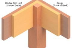
For Single Rim Joist use a 12" long block to permit proper frame spacing.
