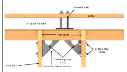
FOR ILLUSTRATED PURPOSES ONLY: SEE ADDITIONAL GUIDELINES PER DECK DESIGN PROFESSIONAL & LOCAL CODE AUTHORITY. INSTALLER IS RESPONSIBLE FOR PREVENTING WATER INTRUSION. TIGHTEN ALL BOLTS & SEAL ALL CAULK. FASTENERS MUST MEET OR EXCEED LOCAL CODE (REC: HDG ASTM 123 HOT DIPPED GALVANIZED OR STAINLESS STEEL) INSTALL ONLY IN PROVIDED, SPECIFIED HOLES. SEE HDGEP.COM FOR SPECS/VIDEOS
